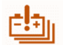
Power battery fault indicator lamp
