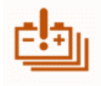
Power battery fault indicator lamp
