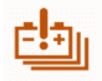
Power battery fault indicator lamp
