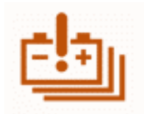
Power battery fault indicator lamp
