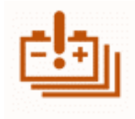
Power battery fault indicator lamp
