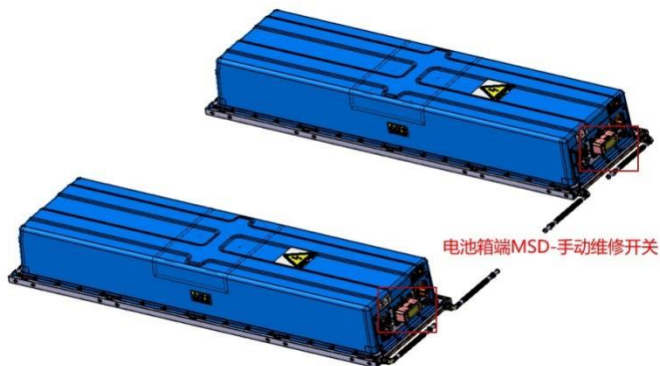
Fig. 1-4 Schematic diagram of high voltage PDU MSD
